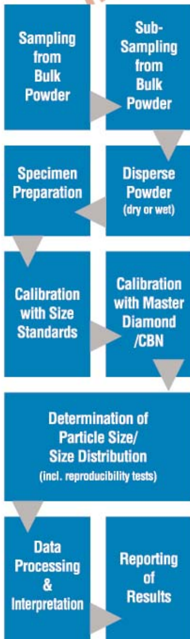
Figure 1 – Flow chart of a general procedure recommended for particle size and size distribution analysis.
